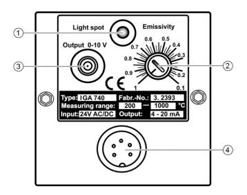
Figure 4: Operating and display elements
