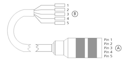
Figure 5: Pyrometer wire connection with configuration
