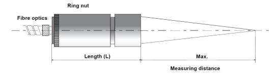
Figure 3: Fibre optic - optical head (fixed optics)
