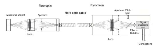
Figure 1: Structure of the pyrometer
