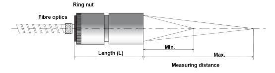
Figure 2: Fibre optic - optical head (vario optics)
