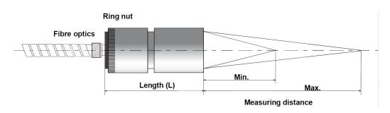
Figure 6: Setting the vario optic head
